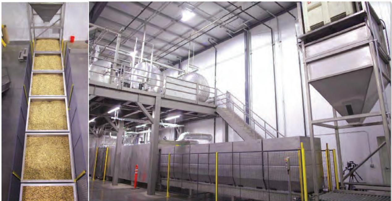
Napason Pasteurisation line of 6 bins showing full bins from the top (left) and bins lined up on the loading platform ready to enter the pasteuriser. Photos courtesy of Poindexter Nut Company. CA, USA
