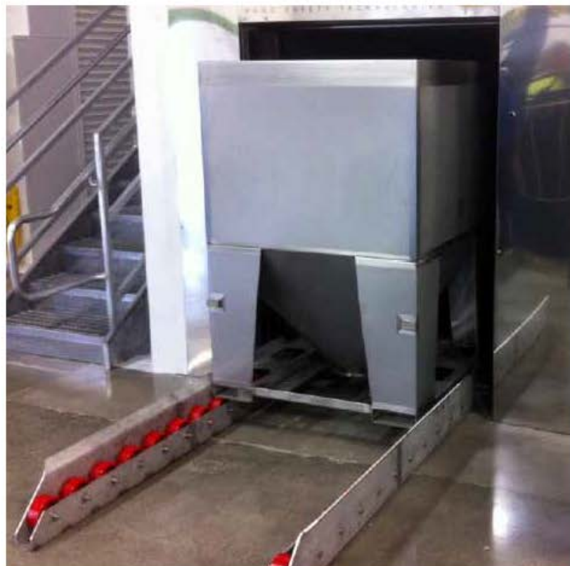
Figure 1. Photograph of loading a 1400lb container of walnuts in the autoclave. This pasteurization unit will hold 6 bins for a total volume of 8400lbs/batch. Total cycle time is 40 minutes including a short pasteurization phase.
